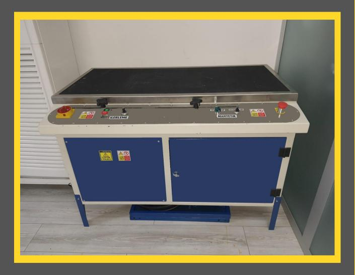
Magnetic presses are used to test fabrics if they can be printed on.
