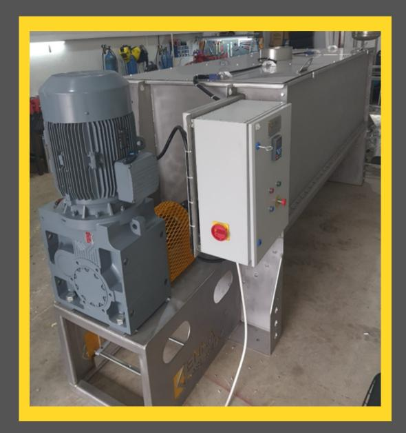
Powder mixers are systems used to mix large quantities of powder products with each other. They are generally used in the detergent industry.
