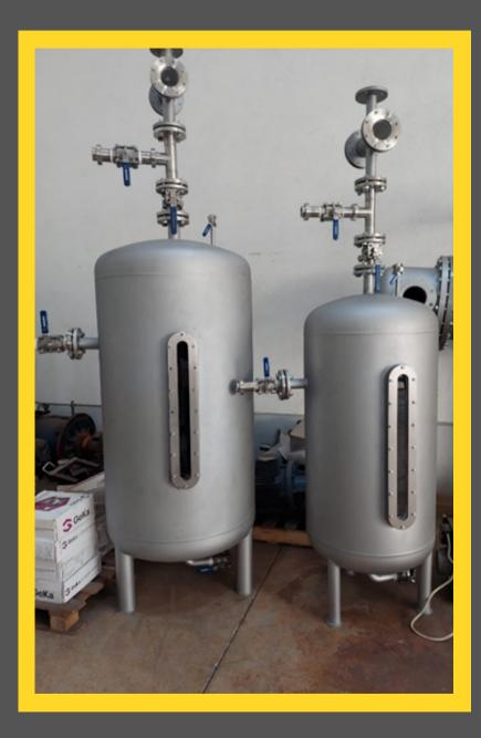
These are tanks where the products that are condensed in the reactors and condensers are accumulated.
