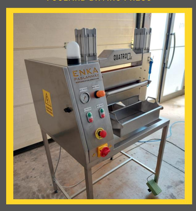
Foular drying presses are designed to dry washed cloth pieces by pressing them between two cylinders.
