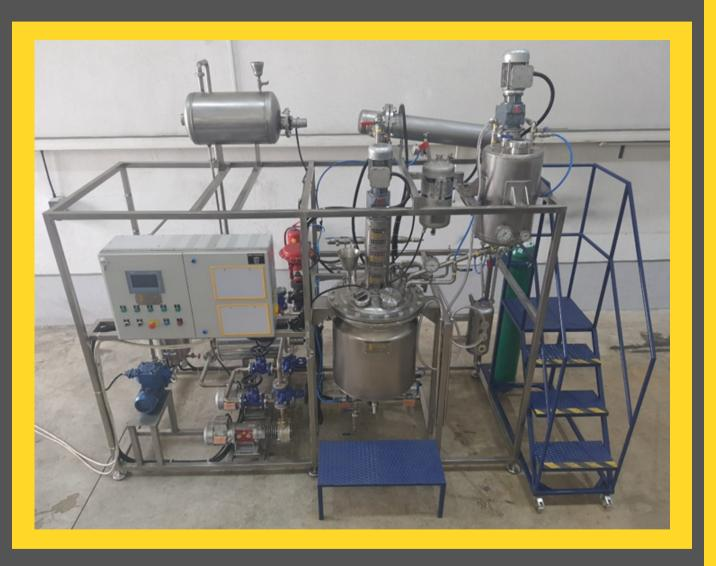
Reactors are tanks in which the ideal environment for the reaction is provided and heating, cooling, mixing processes can be done separately or together.
